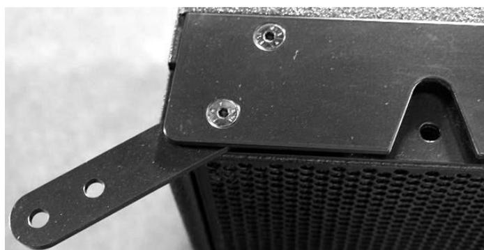
the unit can be secured to the upper speaker system or flying bar. The swing arms on the rear are also used to adjust the orientation, the vertical angle, between the various elements. A label stating the specific holes to be used for achieving a certain orientation is located next to each speaker system.
