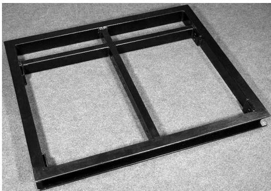
The LA12 (LA12C) has been designed to bear heavy loads and is equipped with two front and two rear end attachment points. There is a central reinforcement bar which is also used for lifting purposes, with six attachment points. The two attachment points at the front and rear of the bar are used to fix the first loudspeaker enclosure's rear and front swing arms.
