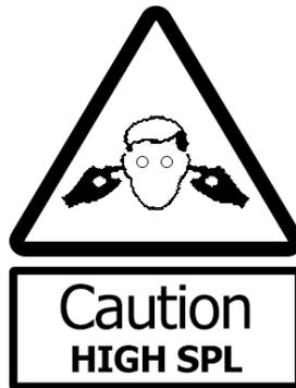
NEXT PXL118 subwoofers are capable of producing extremely high sound pressure levels and should be used with care. Hearing loss is cumulative and can result from levels above 90dB if people are exposed for a long period. Never stand close to loudspeakers driven at high levels.
