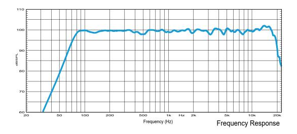
Sensitivity curve of a single LA26 cabinet (Full-Range Operation) using NEXT-proaudio's audio processing. The measurement was made in anechoic environment at 1W@1m.
