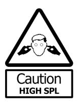
NEXT PXL118 subwoofers are capable of producing extremely high sound pressure levels and should be used with care. Hearing loss is cumulative and can result from levels above 90dB if people are exposed for a long period. Never stand close to loudspeakers driven at high levels.
