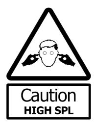
NEXT-proaudio X Series systems are capable of producing extremely high sound pressure levels and should be used with care. Hearing loss is cumulative and can result from levels above 90dB if people are exposed for a long period. Never stand close to loudspeakers driven at high levels.
