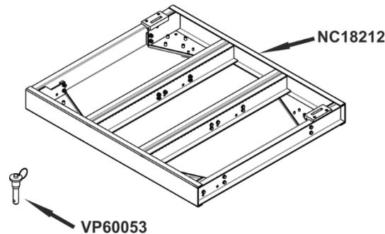
The stacking can be accomplished directly on the ground up to six units or on top of the NEXT LAS418 Subwoofer up to four units. The subwoofer has grooves to accommodate the plastic feet of the rigging frame. When on the ground, wheels can be mounted to the rigging frame prior to assembly, to make movement easier.
