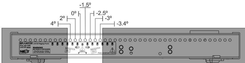
The greyed-out areas are not to be used. One can now continue to do the rest of the assembly with the elements as needed **up to a maximum of 6 enclosures.**
